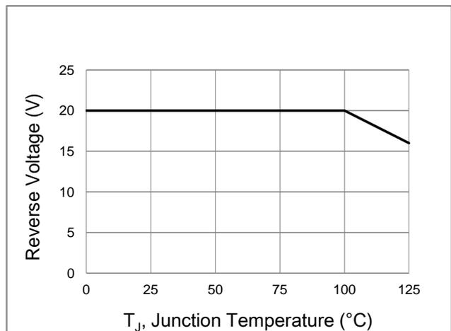
Fig. 4. Operating Temperature Derating Curve
