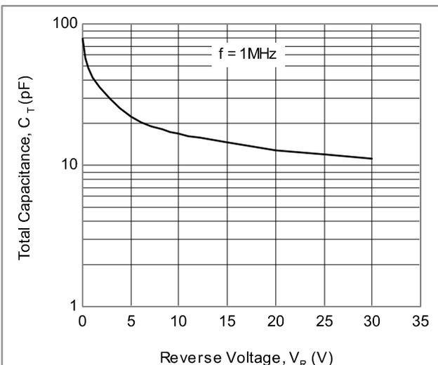
Fig. 3. Typical Capacitance
