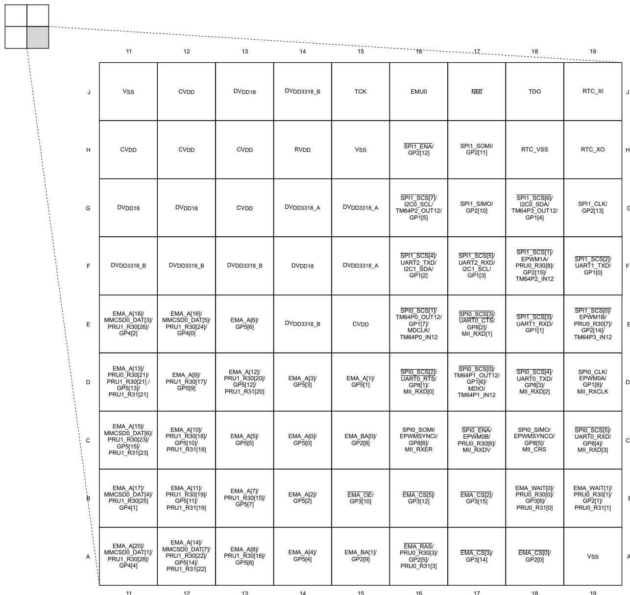
Figure 3-5. Pin Map (Quad C)
