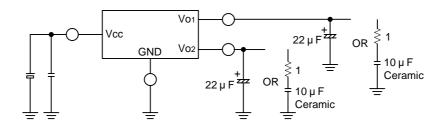
TEST CIRCUIT FOR EACH CONDITION
