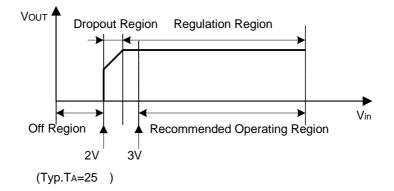
For proper regulation, this device must be operated in the Recommended Operating Region shown above.
