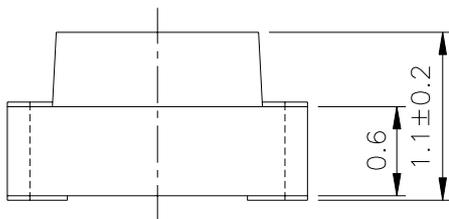
For reflow soldering (Propose)
