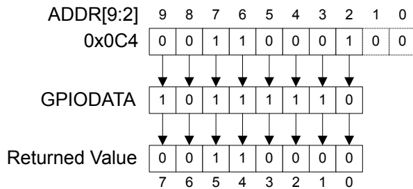
Figure 8-3. GPIODATA Read Example
