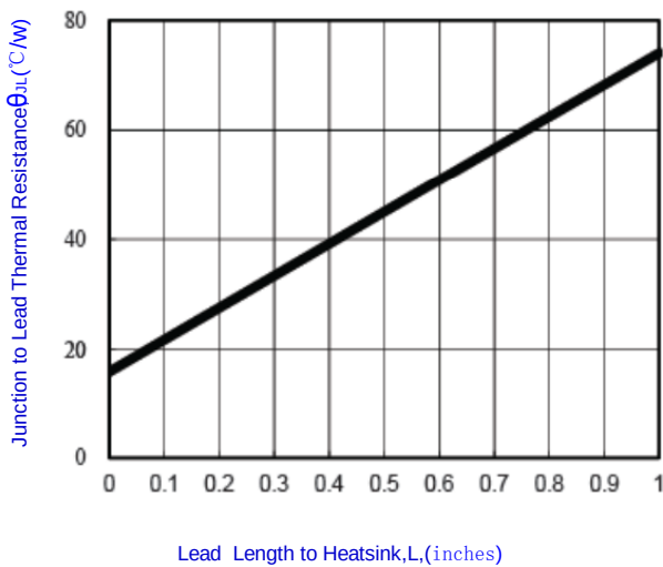
Fig.3- Typical Thermal Resistance V.S. Lead Length
