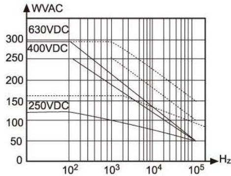
Working Voltage DC&AC vs. Frequency
