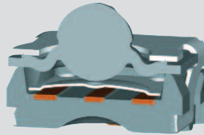
Sectional view of keyswitch
