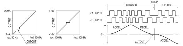
Forward Rotation: Phase A leads the Phase B by 90 degrees. Reverse Rotation: Phase A lags behind Phase B by 90 degrees.
