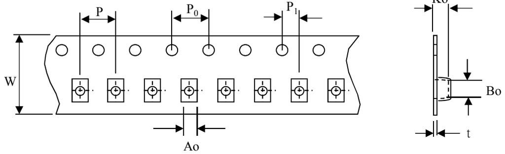
(Dimensions in mm; Tolerance : ±0.1)
