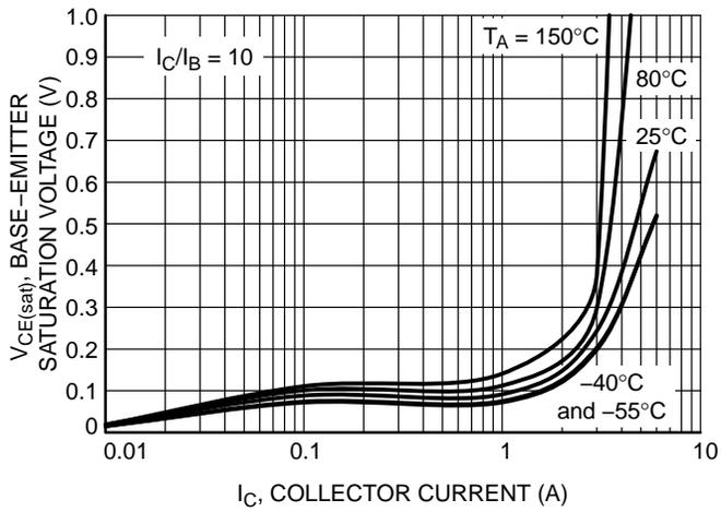
Figure 7. Collector Emitter Saturation Voltage vs. Collector Current
