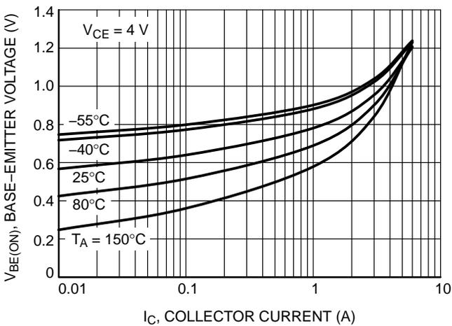
Figure 5. Base Emitter Voltage vs. Collector Current
