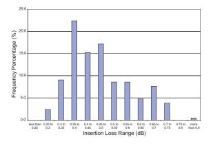
Typical robustness of the design — ~0.15 dB attenuation change after 10 million cycle dynamic load test on the normally closed VOA
