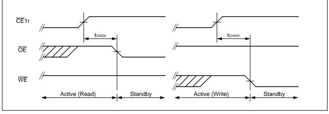
Note : Both t<sub>CHOX</sub> and t<sub>CHWX</sub> define the earliest entry timing for Standby mode. If either of timing is not satisfied, it takes t<sub>RC</sub> (Min) period for Standby mode from CE1r Low to High transition.
