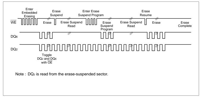
• RY/BY Timing Diagram during Program/Erase Operation Timing Diagram
