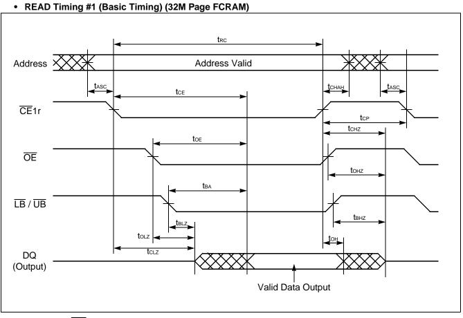
Note : CE2r and  $\overline{\text{WE}}$  must be High for entire read cycle.
