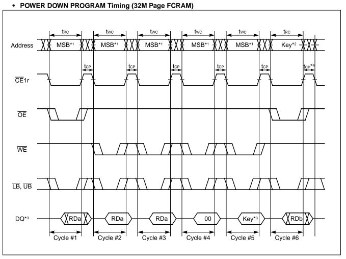
\*1 : The all address inputs must be High from Cycle #1 to #5. The address key must confirm the format specified in "■ 32 M FCRAM CHARACTERISTICS for MCP 1. Power Down Program Timing (32 M Page FCRAM) ". If not, the operation and data are not guaranteed.
