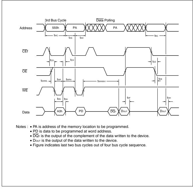
Alternate WE Controlled Program Operation Timing Diagram
