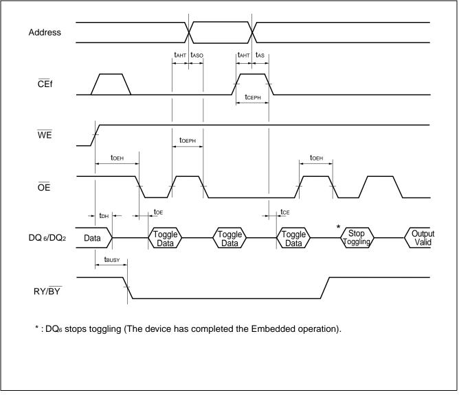
• AC Waveforms for Toggle Bit I during Embedded Algorithm Operations
