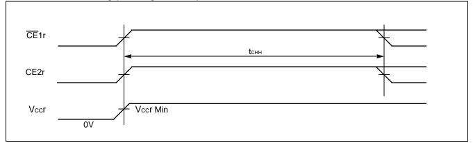
Note : The tCHH specifies after Vccr reaches specified minimum level and applicable both TE1r and CE2r.
