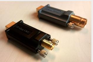
In addition to the long-haul fully duplex data transmission, power can be transmitted simultaneously from the host side to a target (such as camera or hard drive) over the coax cable.
