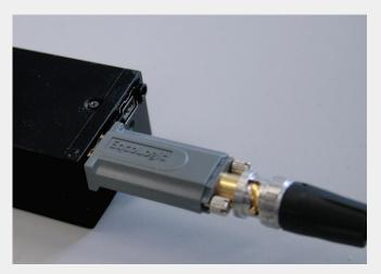
When using the dongles, customers can determine the best cable lengths for their applications. The EqcoLogic transceiver contains an equalizer that is fully adaptive and adjusts for various cable lengths as well as age and environmental conditions like temperature, without any need for programming. The dongles have a standard 1394b 9-pin connector on one end and a 75 $\Omega$  BNC or 50 $\Omega$  SMA connector on the opposite end.
