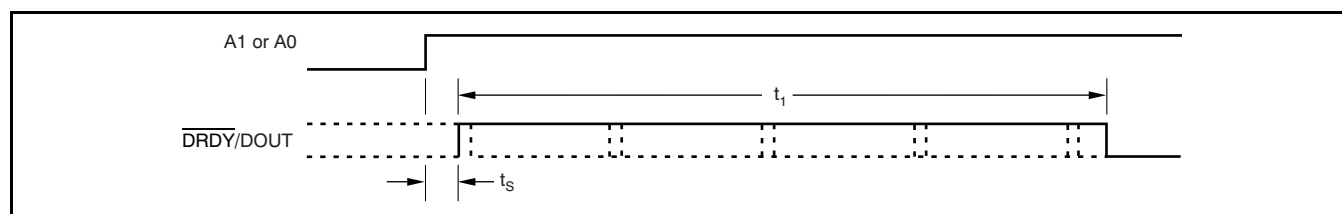
Figure 32. Example of Settling Time After Changing the Input Multiplexer
