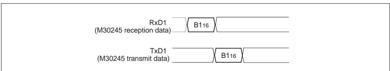
Figure 1.196. Timing of baud rate 19200
