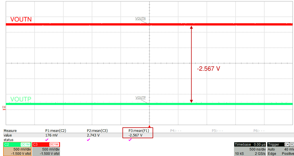
Figure 7-5. Typical Failsafe Output of the AMC3301-Q1
