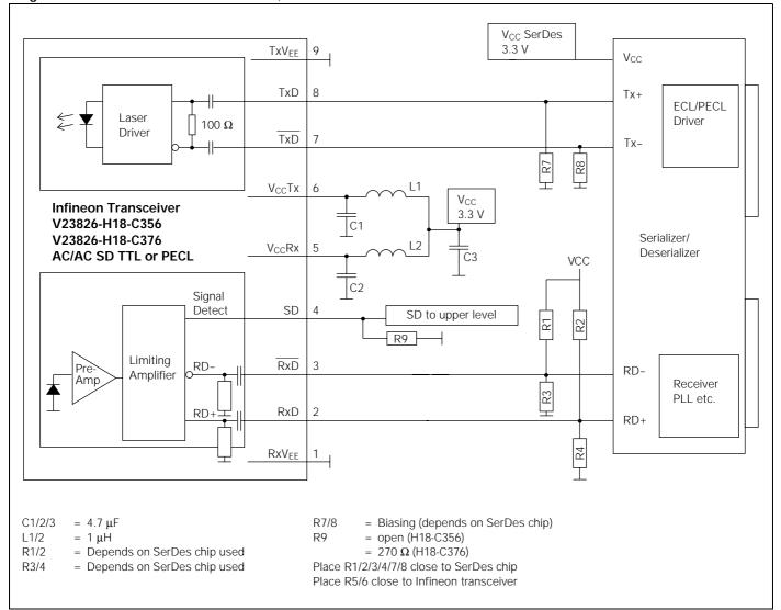
Values of R1/2/3/4 may vary as long as proper 50  $\Omega$  termination to  $V_{EE}$  or 100  $\Omega$  differential is provided. The power supply filtering is required for good EMI performance. Use short tracks from the inductor L1/L2 to the module  $V_{CC}Rx/V_{CC}Tx.$  Further application notes for electrical interfacing are available upon request. Ask for Appnote 82.
