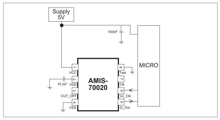
The power supplies of the chip need to be properly decoupled. This means that at least one external capacitor CDD must be connected in between VSS and VCC.
