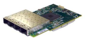
integrated Gigabit Ethernet Media Access Control (MAC) and SFI Interface. In addition to managing MAC and PHY Ethernet layer functions, the controller manages PCI Express packet traffic across its transaction, link, and physical/logical layers. Using hardware acceleration, the controller offloads tasks from the host, such as TCP/UDP/IP checksum calculations and TCP segmentation.
