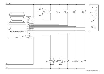
Protective field switching between two S300 with static and dynamic inputs
