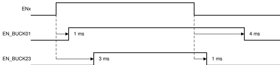
Figure 16. Typical Start-Up and Shutdown Sequencing
