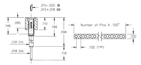
**Description:** Interconnect Socket Elevated Strip Socket Accepts .015" - .025" (0,38 - 0,635 mm) dia leads Single Row Through Hole
