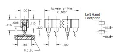
Interconnect Socket Surface Mount Socket Accepts .015"- .025" (0,38 - 0,635 mm) dia leads Single Row Surface Mount **Plating Code:** 43 Shell Plating: 200 µ" Tin (matte finish) over 100 µ" Nickel
