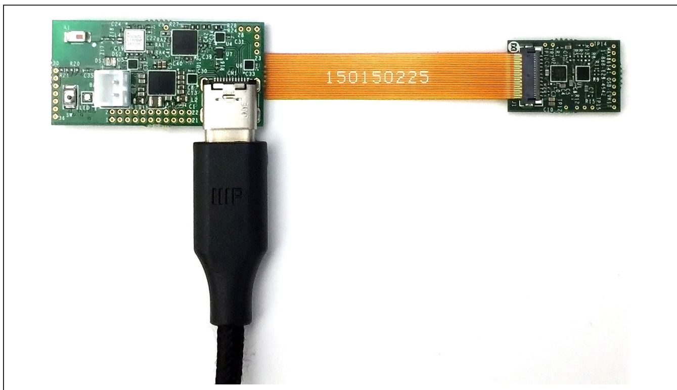
Figure 11. Hardware Setup (MAX86141 EVSYS Micro PCB)
