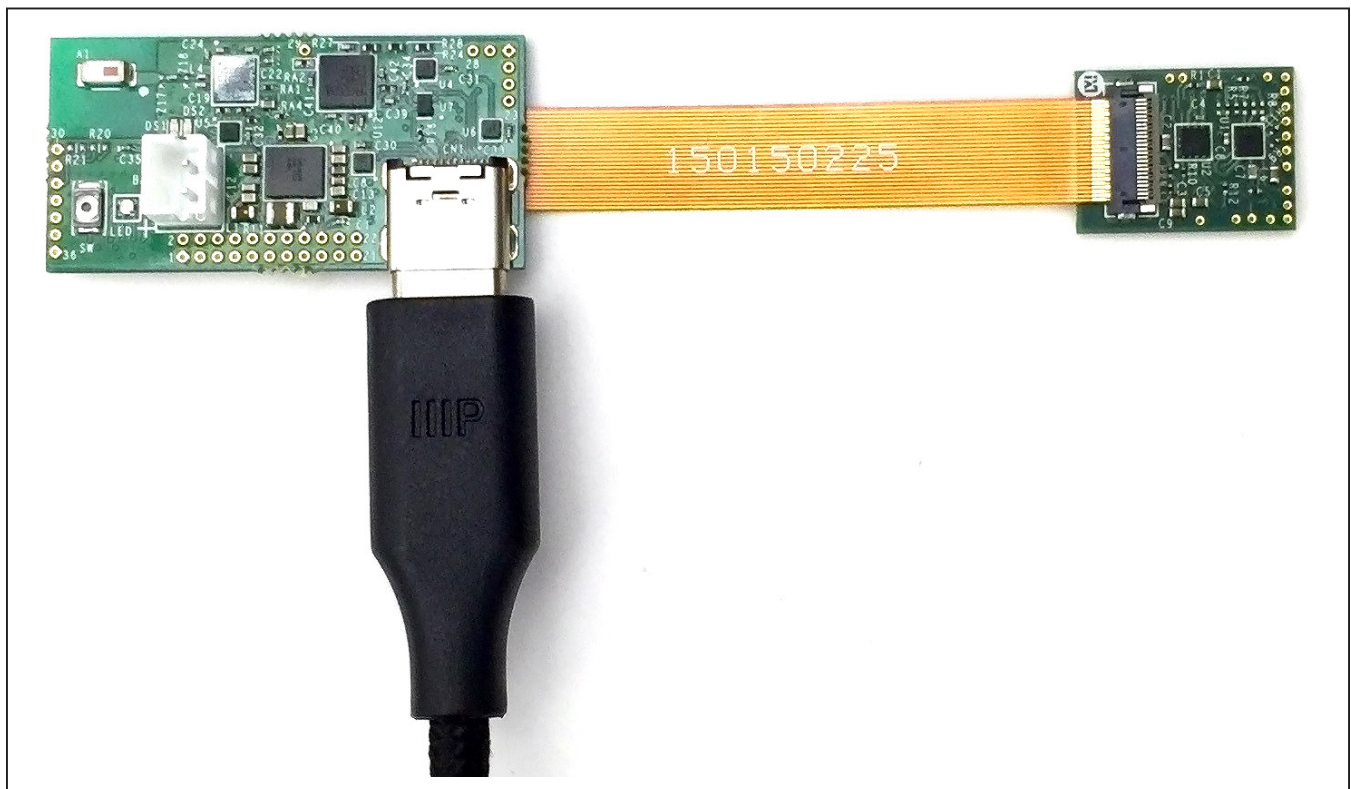
Figure 9. Hardware Setup (MAX86140 EVSYS Micro-PCB)
