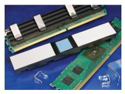
Gap Pad® HC 1000 is an extremely conformable, low-modulus polymer that acts as a thermal interface and electrical insulator between electronic components and heat sinks. The "gel-like" modulus allows this material to fill air gaps to enhance the thermal performance of electronic systems. Gap Pad® HC1000 is offered with removable protective liners on both sides of the material.
