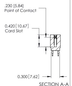
725 Series Ultra-Mate Card Edge Connector - Press Fit
