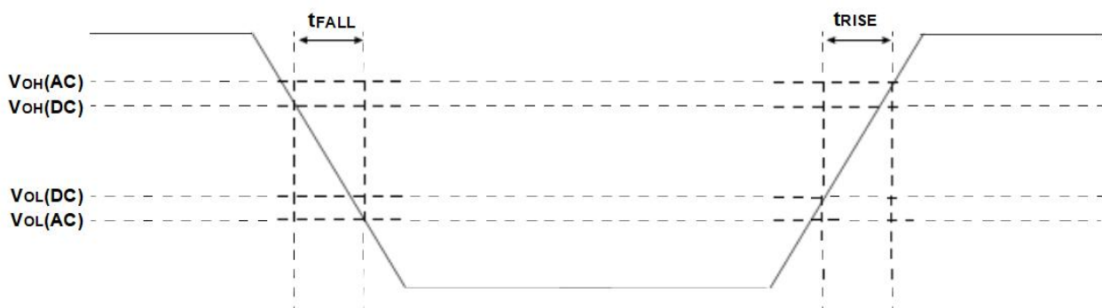
Figure 5. t_{RISE} and t_{FALL} Definition for Output Slew Rate
