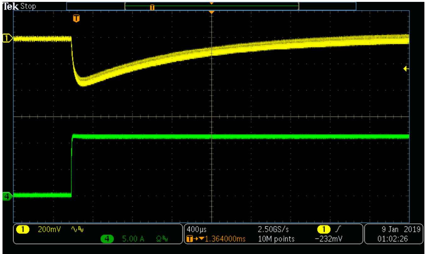
Figure 14. Load Step Up With 40 V IN
