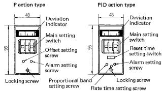
Note) The controller enclosure is the same in shape and dimensions as the output converter enclosure.
