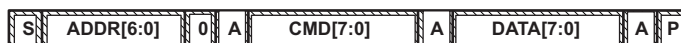
Figure 7. Attempt To Write a Read-Only Address (Nack After Data Sent By Master)
