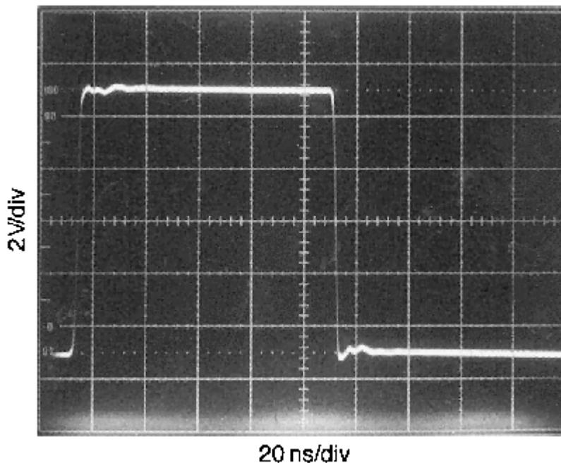
**Figure 48. Properly Terminated Signal**
