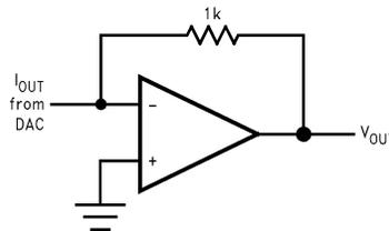
**Figure 50. I-to-V Converters**
