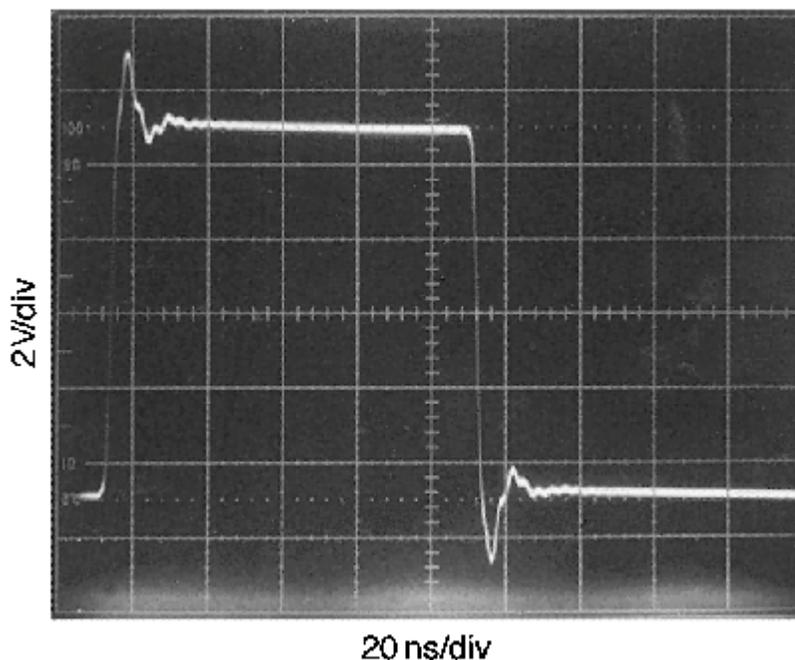
**Figure 49. Improperly Terminated Signal**
