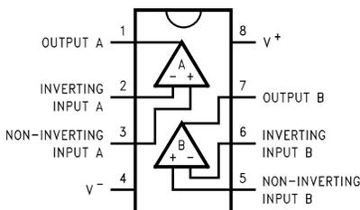
**Figure 1. Top View 8-Pin**
