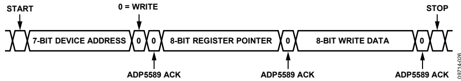
Figure 27. I 2 C Single-Byte Write Sequence
