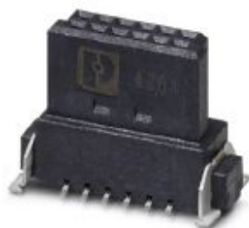
SMD female connector, Nominal current at 20 °C: 1.4 A, Test voltage: 500 V AC, number of positions: 32, pitch: 1.27 mm, color: black, contact surface: Gold, mounting: SMD soldering
