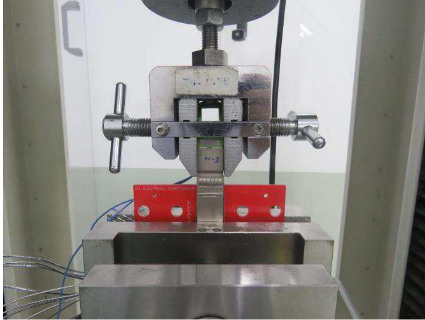
Figure 4 – Typical Cage Latch Axial Retention Test Setup
