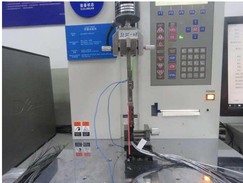
Figure 5 – Typical Mating Force Test Setup
