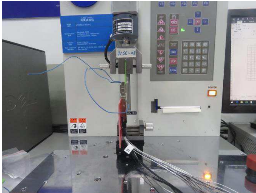
Figure 6 – Typical Unmating Force Test Setup
