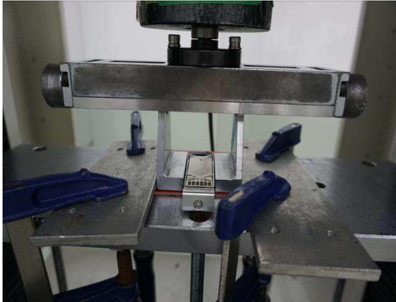
Figure 8 – Typical Cage Compliant Pin Retention force Test Setup
