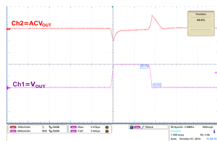
Figure 38: Load transient ( V_{OUT} = 5\text{ V} )
