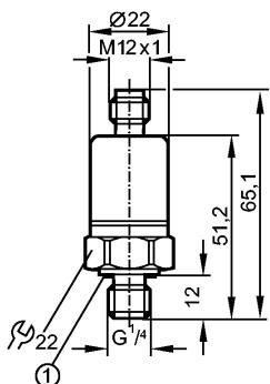
1: sealing NBR / DIN 3869-14
