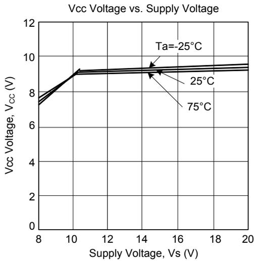
Vcc voltage generates by the constant voltage circuit in IC. This is measured not by M54123L but by a special element.
