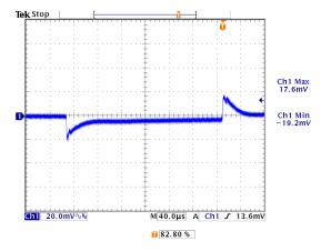
Figure 24: Transient response, 0.9V/20A, Ch1: Vo
