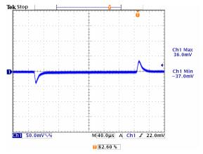
Figure 22: Transient response, 1.5V /20A, Ch1: Vo
