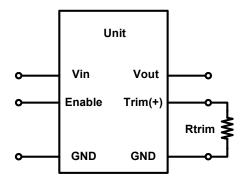
Figure 27: Trimming Output Voltage
