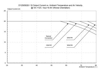
Figure 39: Output current vs. ambient temperature and air velocity @Vin=12V, Vout=0.9 V (Worst Orientation)
