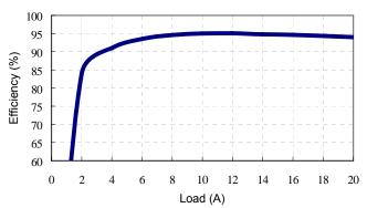
Figure 1: Converter efficiency vs. output current (5.0V output voltage, 12V input)
