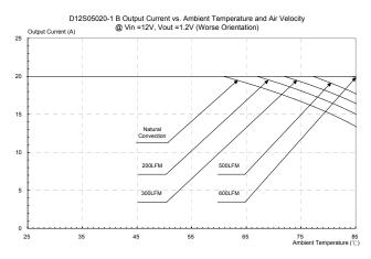
Figure 37: Output current vs. ambient temperature and air velocity @ Vin=12V, Vout=1.2V (Worst Orientation)
