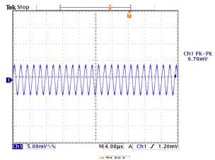
Figure 8: Output ripple & noise at 12Vin, 3.3V/20A out
