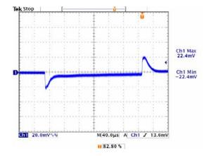
Figure 23: Transient response, 1.2V /20A, Ch1: Vo
