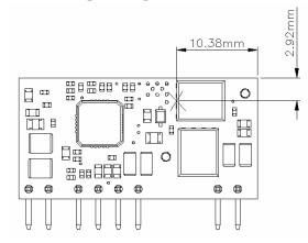
**Figure 31:** Temperature measurement location\* The allowed maximum hot spot temperature is defined at 125  $^{\circ}$ C
