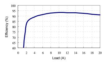
Figure 2: Converter efficiency vs. output current (3.3V output voltage, 12V input)
