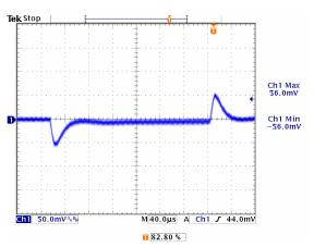
Figure 21: Transient response, 2.5V /20A, Ch1: Vo
