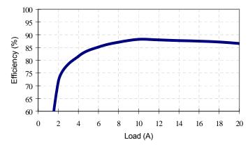
Figure 4: Converter efficiency vs. output current (1.5V output voltage, 12V input)
