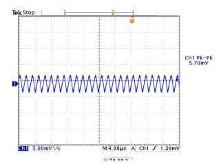
Figure 10: Output ripple & noise at 12Vin, 1.5V/20A out
