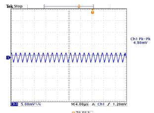
Figure 12: Output ripple & noise at 12Vin, 0.9V/20A out
