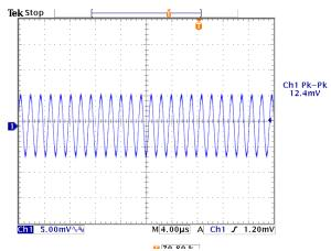
Figure 7: Output ripple & noise at 12Vin, 5.0V/20A out
