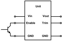
Figure 25. Enable Input drive circuit for D12S05020
