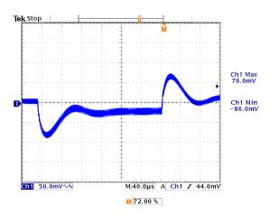
Figure 19: Transient response, 5.0V /20A, Ch1: Vo
