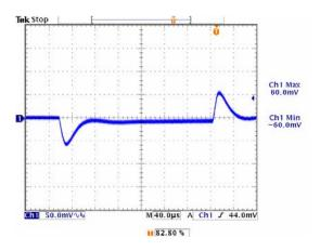
Figure 20: Transient response, 3.3V /20A, Ch1: Vo
