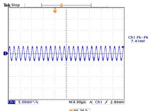
Figure 9: Output ripple & noise at 12Vin, 2.5V/20A out
