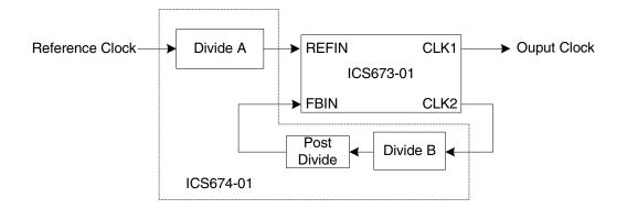
If the reference is in the kHz range, for example 8 kHz, the following configuration may be more typical:
