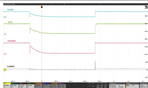
Figure 9-5. Response to ISO 7637-2 Pulse 1
