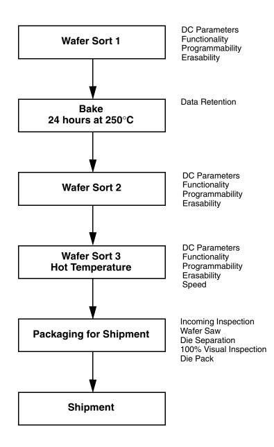
Figure 1. AMD KGD Product Test Flow
