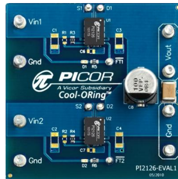
Figure 1: PI2126-EVAL1 Evaluation Board (1.8" x 1.8")
