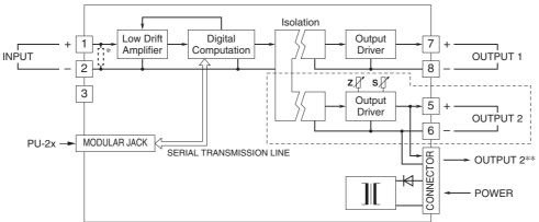
Input shunt resistor incorporated for current input.
