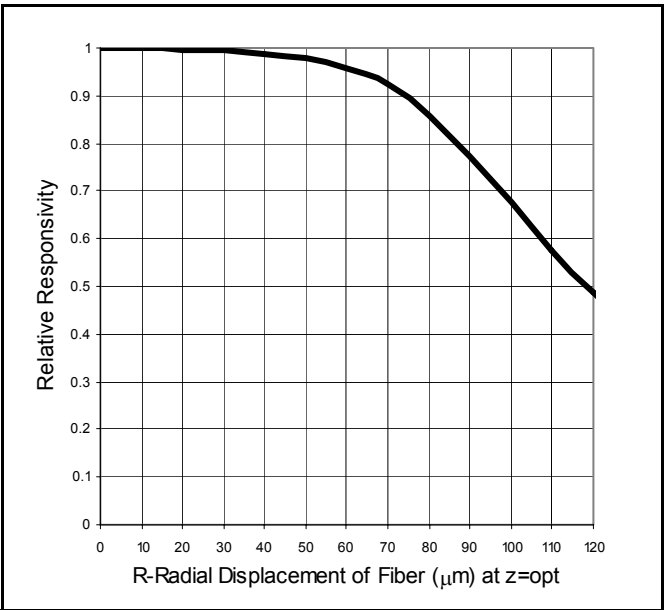
Figure 5 - Typical Responsivity vs Radial Displacement for a Multimode Fiber
