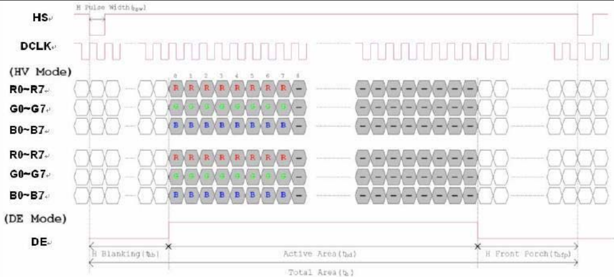
1 Horizontal input timing diagram.
