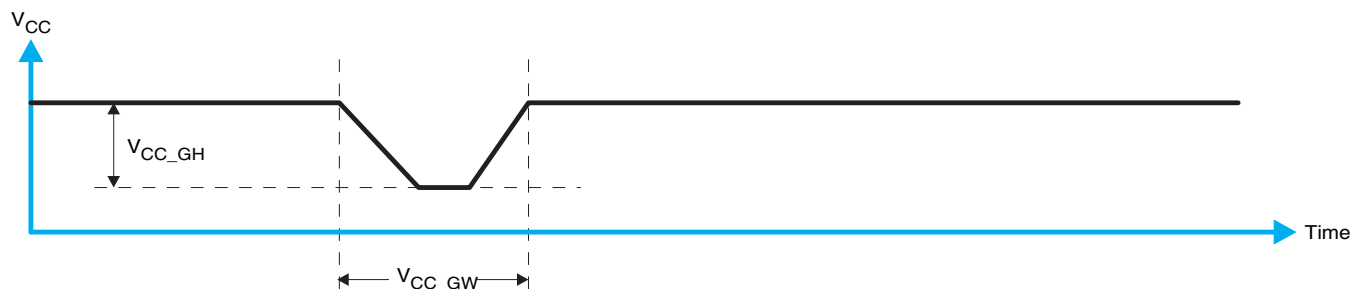
Figure 25. Glitch Width and Glitch Height
