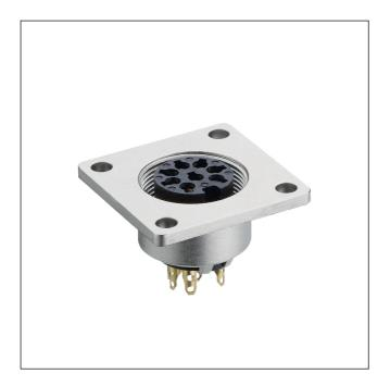
Flange chassis socket acc. to IEC 61076-2-106 and AISG specification, IP 68, with threaded joint and solder terminals, for front mounting
