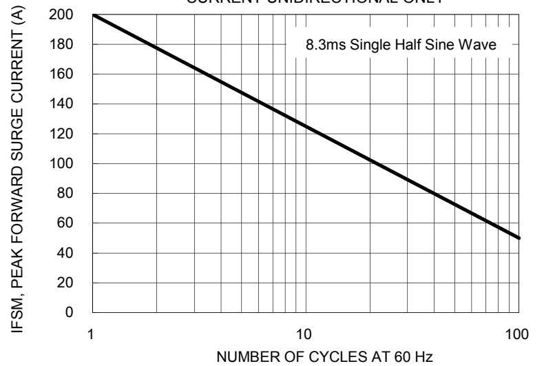
FIG. 4 MAXIMUM NON-REPETITIVE FORWARD SURGE CURRENT UNIDIRECTIONAL ONLY
