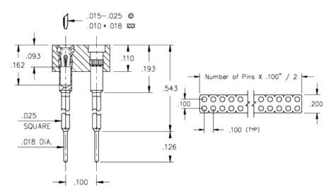
**Description:** Interconnect Socket Wrapost with Solder Tail Socket Accepts .015" - .025" (0,38 - 0,635 mm) dia leads Double Row Through Hole Plating Code: Shell Plating:
